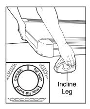
position. Lower the treadmill, making sure that the incline leg is resting flat on the floor.
